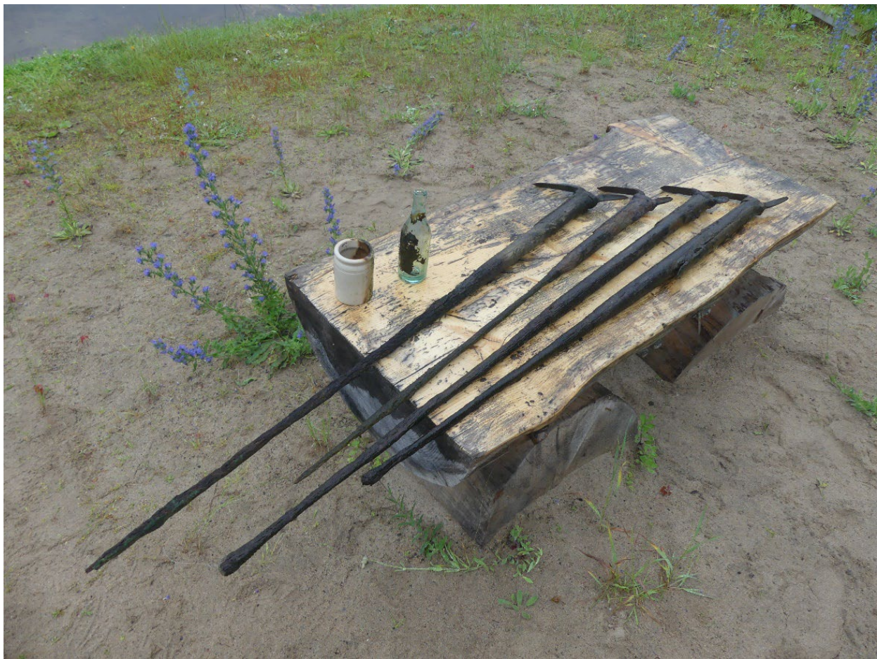
Remnants from ice harvesting on Moody Pond – Pick Poles (also known as pike poles)
