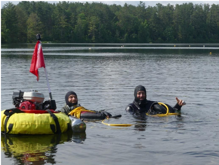
Divers utilizing a Hookah floating air compressor and buoys marking EWM plants in the background - Photo: Guy Middleton
