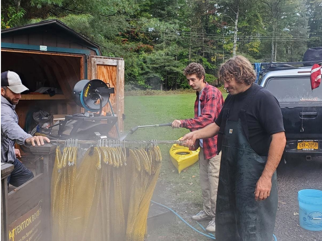
Equipment sanitization utilizing the USF's hot water / high pressure decontamination unit at Upper Saranac Lake– Photo: Guy Middleton
